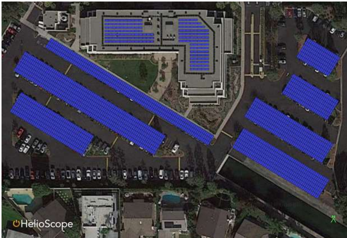
Figure 53: CSULB Foundation Building – Potential PV Site Plan
