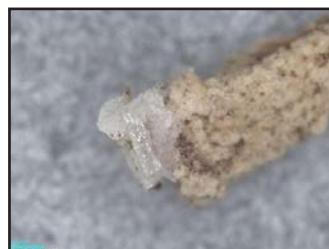
WOOD COVERED IN CARBONATE AND A POSSIBLE CALCITE GROWTH ON THE END
