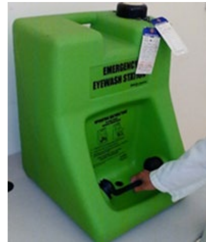
GREEN: grasp black strap and pull to remove covers
